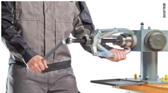
Figure 2 Use of the three-arm extractor PULLER-3ARM
