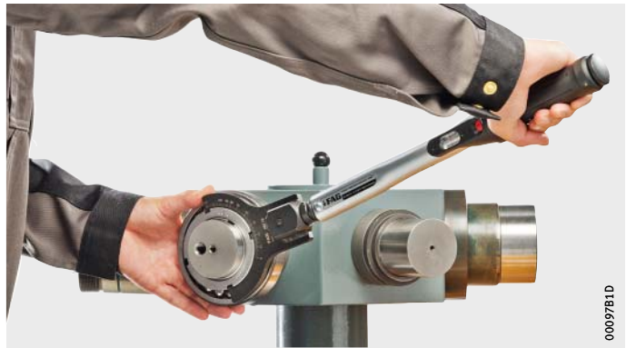
Figure 3 Use of the double hook wrench LOCKNUT-DOUBLEHOOK
