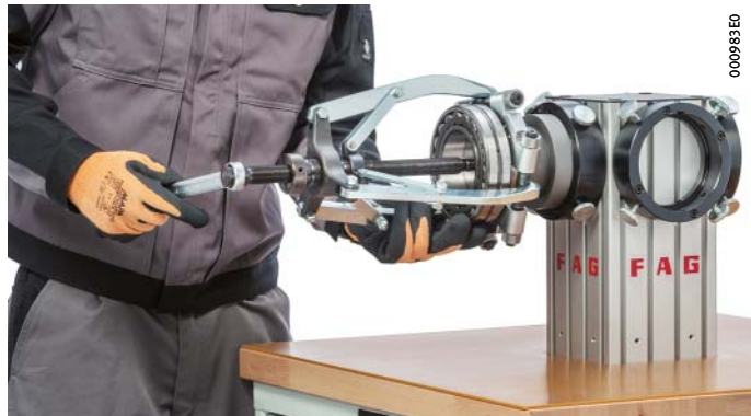
Figure 2 Use of the three-section extraction plate PULLER-TRISECTION
