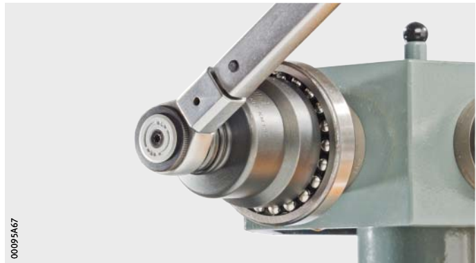
Figure 2 Use of the socket LOCKNUT-SOCKET
