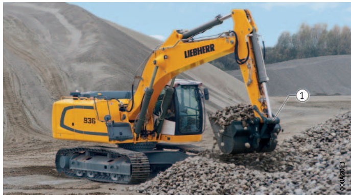
Figure 5 Application example with high wear load: spherical plain bearings in excavator
