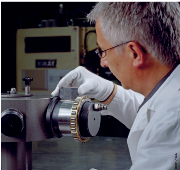
Figure 5 Measuring the spacing from the shaft shoulder
