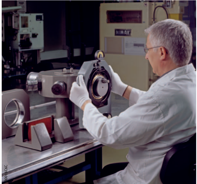
Figure 4 Positioning the enveloping circle gauge
